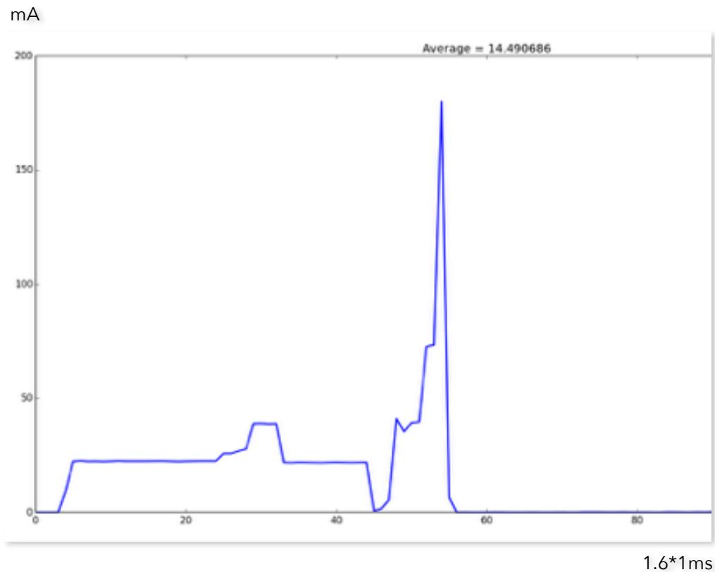
During one deep-sleep cycle, the chip will wake up at a specific time and begin transmit data, and then enter deep-sleep mode again. Implementation of this low-power solution can be realized by decreasing the time period and lowering the current.
